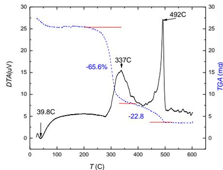
**Fig. 47** TG DTA thermogram of extrudate obtained from the mixture with a ratio starch / glycerol / water [% by weight] 68/17/15
