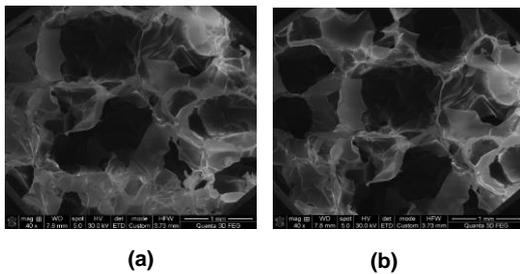
**Fig.46** SEM images of the extrudate obtained from mixtures with a ratio of starch / glycerol / water [% by weight]: 68/17/15 (a) = cross section; (b) = in longitudinal section
