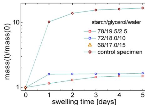
**Fig.1.** The normalized mass absorbed during of 5 days by the 3 packaging samples with constant ratio of 4: 1 starch / glycerol compared with the standard sample
